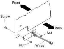
Figure 27 - Switch Plate and Wiring Harness (Switch Plate and Orientation May Vary Depending On Model)
